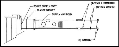
Figure 14. Supply Manifold Assembly
